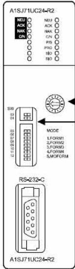
1. Set the communication protocol form on Mode Setting Rotary Switch as below.
