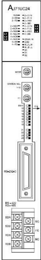
1. Set the communication protocol form on Mode Setting Rotary Switch as below.
