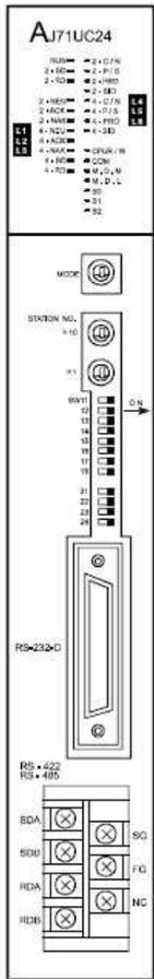
1. This sets communication protocol form on Mode Setting Rotary Switch as below.
