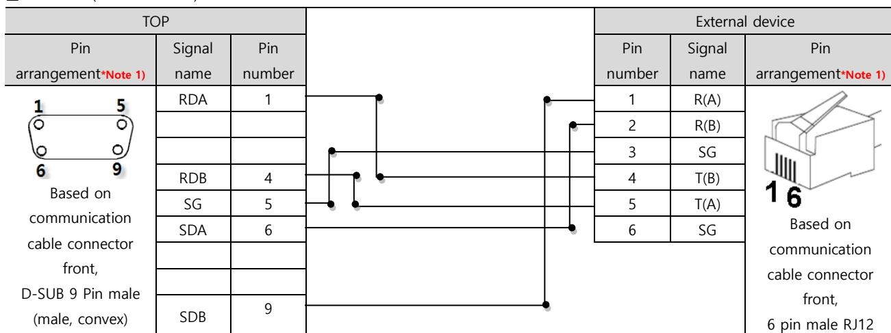
\*Note 1) The pin arrangement is as seen from the connecting side of the cable connection connector.
